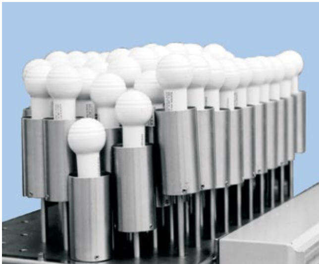
Figure 8: 3-D heating panel for laminating door trims
