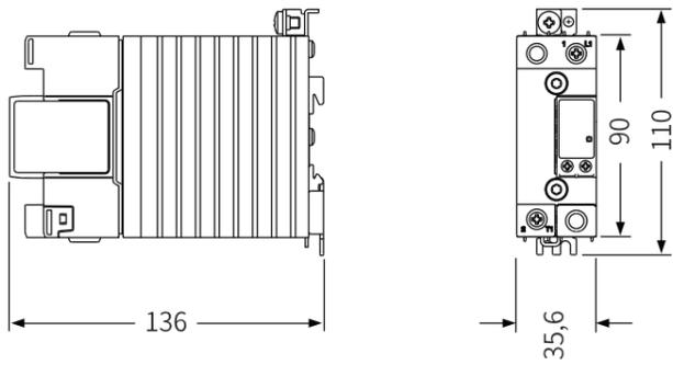
Mounting dimensions and radiator dimensions ( ) in mm
