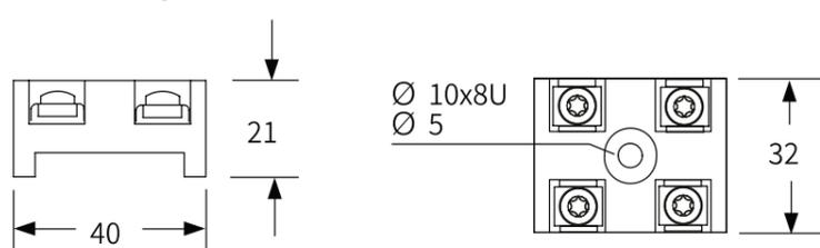
Mounting dimensions and radiator dimensions ( ) in mm
